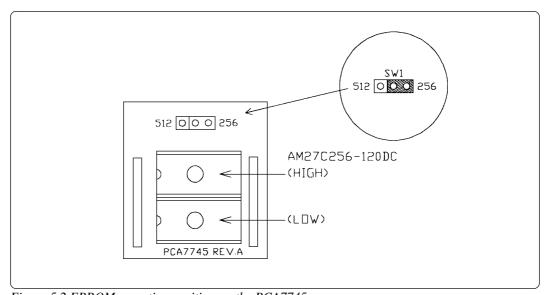
Figure 5.2 EPROM mounting position on the PCA7745
